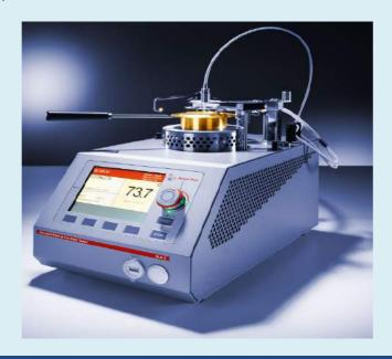
Our laboratory is equipped with Pensky Marten Closed Cup Apparatus for Flash Point Test
